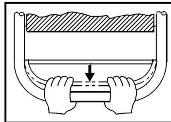
7. To stop Evacu-Trac on the stairs, slowly release the Brake Release Bar.
