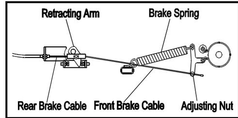
To check this, lay the open Evacu-Trac on its side. Locate the Front Brake Cable. It should have approximately 19 mm (3/4 in) of slack, when measured vertically from the reference point shown in the drawing to the right.
