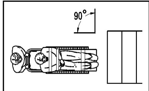
5. Push Evacu-Trac forward until the Front Auxiliary Wheels drop off the top step. At this point Evacu-Trac will stop. To prevent Evacu-Trac from immediately beginning to descend the stairs, release your grip on the Brake Release Bar. This will engage the Track Parking Brake until you are ready to descend. Lift the handle and tilt Evacu-Trac to the angle of the stairs.
