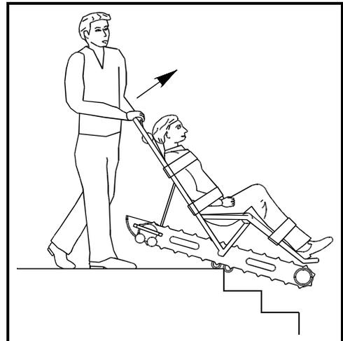
6. To descend the stairs, squeeze the Brake Release Bar. To slow the descent speed, if desired, simply loosen your grip on the Release Bar. This will partially engage the Brake.
