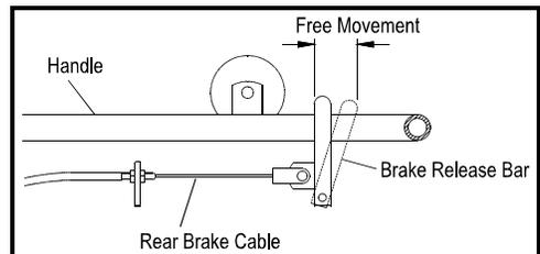
2. When you squeeze the Brake Release Bar it should travel until it just makes contact with the lime green Handle. This will allow you to comfortably hold Brake Release Bar in its released position when pushing Evacu-Trac on flat surfaces or descending a stairway.
