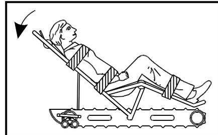
2. Then squeeze the Brake Release Bar with both hands. This will deploy the Front Auxiliary Wheels, making Evacu-Trac easier to push.
