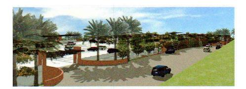
The parking structure will take advantage of the hillside contours. It will be five levels on the west side and decrease to only two levels on the east side to protect neighboring residents' sightlines. It will provide 2,085 spaces. Because it will be built on an existing lot with 435 spaces, the total addition of spaces is 1,650. Temporary lot M was developed to ease the loss of spaces during construction.
