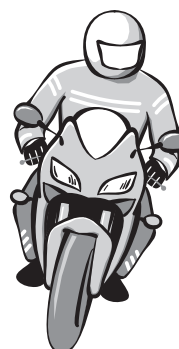
Front wheel momentarily out-tracks away from turn, causing motorcycle to begin leaning in turn direction.
