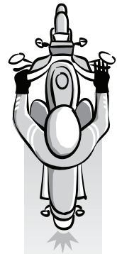
Proper braking. Neither wheel is locked and motorcycle is in alignment.
